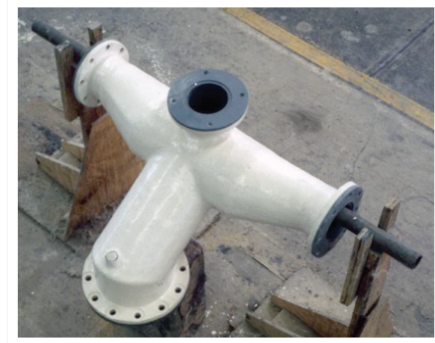
Lined Custom Piping
